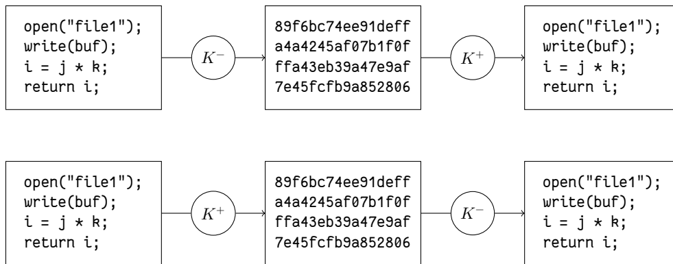
Figure 2.6: Properties of asymmetric encryption. Note the switched use of public and private keys.
